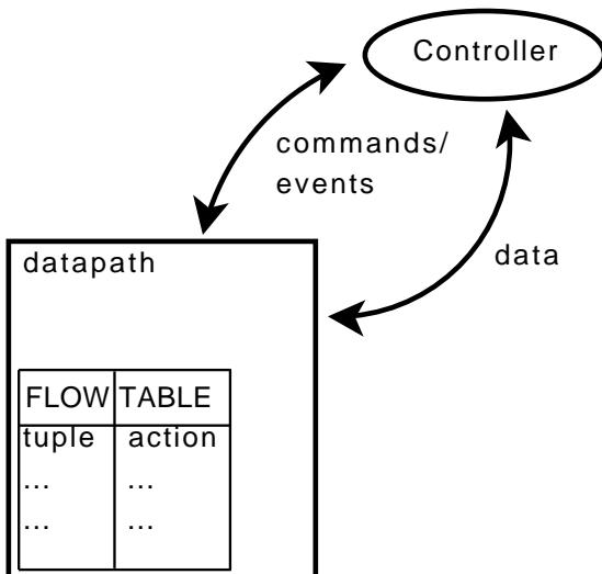
Figure 1: A virtual switch architecture.
