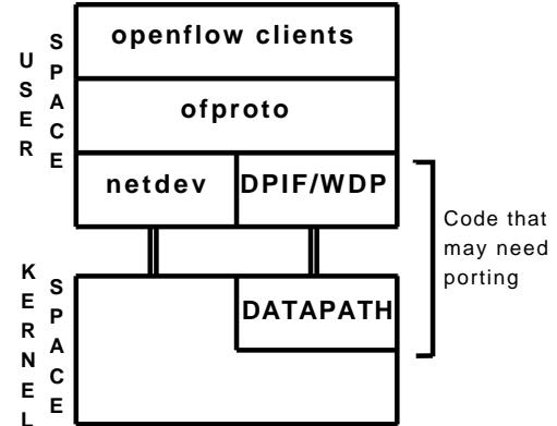
Figure 2: A virtual switch architecture.
